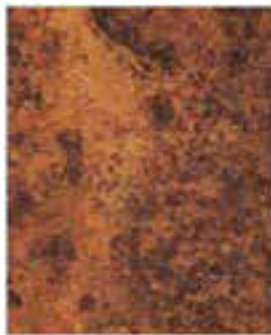
Steel where pitting and complete rusting has occurred
