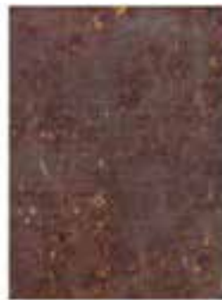
Steel where the mill scale has started to flake and light rusting occurs
