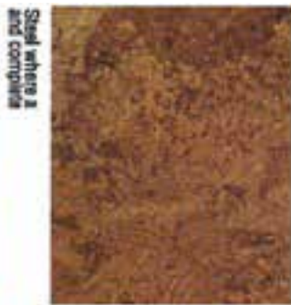
Steel where all the mill scale has flaked off and complete rusting has taken place
